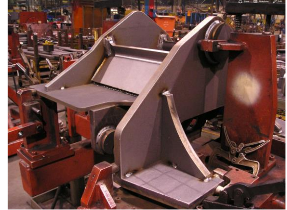
Chassis (Weldment Assemblies)
